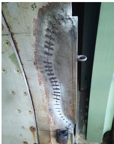
Figure 3 Example of cold stitching
