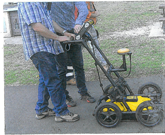
Field GPR unit with GPS locator
